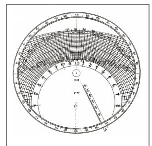
Fig. 1 The stereographic dial or horizontal instrument according to William Oughtred – a stereographic projection of the celestial sphere onto a horizontal plane. When used as a sundial, this instrument not only indicates the time but it also solves most astronomical problems relating to the sun's position in the sky.
